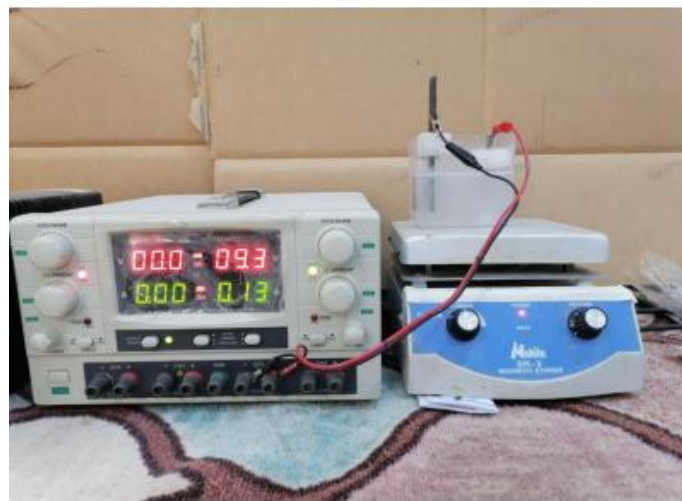
Figure 1: The \text{Al}_2\text{O}_3/\text{ZnO} Nano composite is prepared using an electrochemical method.
